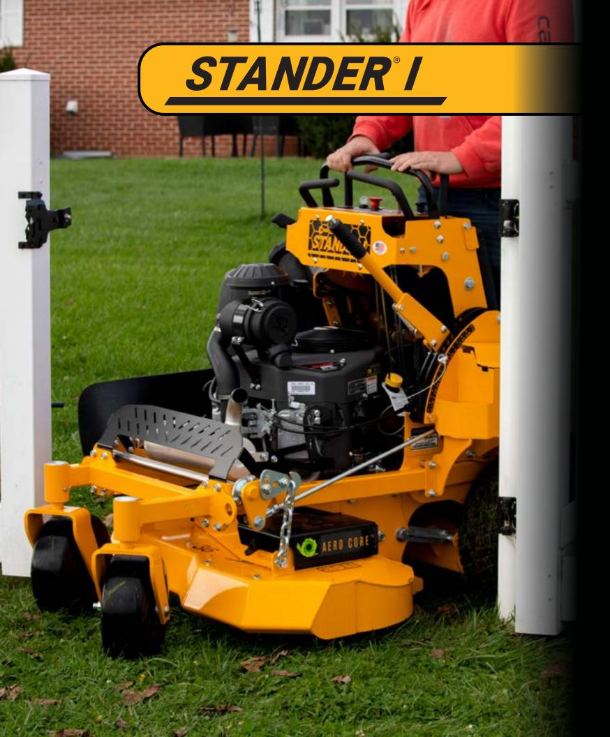
**The STANDER INTENSITY** is just that, it's our most intense and heavy-duty narrow mower with 36" and 42" decks. Great for continuous commercial use on smaller properties and tight areas. It's much more than a trim mower with many years of proven durability.
